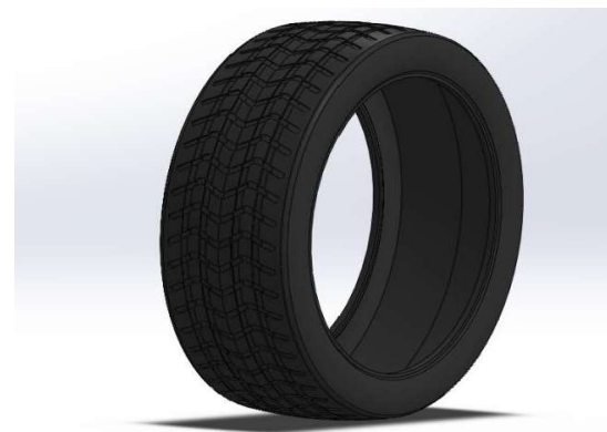
Fig.2 Linear Groove (Symmetrical Type A)
