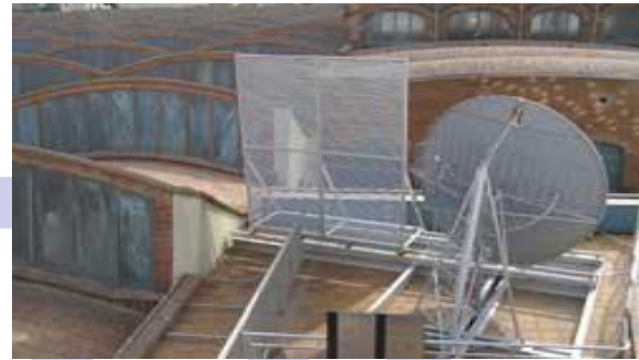
Fig.3 A Scheffler reflector being used as a solar cooker to cook food by concentrating the sunlight. Credit Alamy stock Photo
